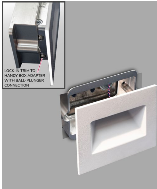
Step 5- Connect low voltage driver wires to step light (assure black to black and red to red and wires are not pinched). Check electrical connection. Insert trim to Handy Box adapter. You will hear a "click" when trim ball plungers engage with adapter (see detail image above)
