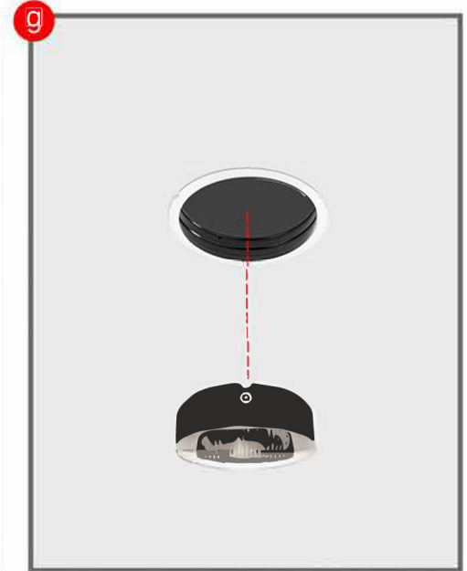
Step G- Position trim to face wall (See below for proper trim position.).
