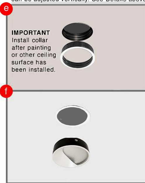
Step E- Flanged collar should be installed after painting, wood, metal ceiling has been prepped. Screw flanged collar into housing. Step F- Slide lamp assembly into collar.
