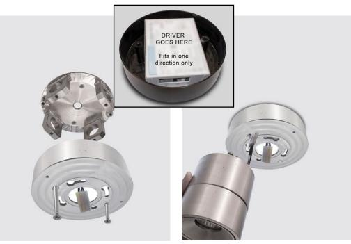
Step 2- Attach Lutron Junction Mounting Driver Box to ceiling plate with #8-32 counter sink screws (Screws supplied by SLI). Driver must be installed before installing Lutron driver box to ceiling.
