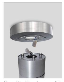
Step 4- Align (4) housing pins on fixture to Lutron Driver Box (4) keyway slots. Push housing into Driver Box while twisting clockwise. (See step 5 for linking mechanism)
