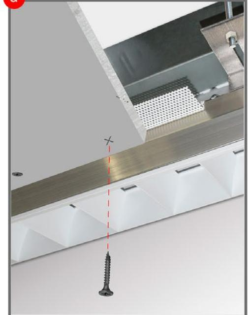
**Step D-** GWB goes around plaster frame and housing, use factory edge against plaster frame. Fasten frame to GWB with sheetrock screws that anchor into perforated metal tabs attached to Ultrim frame.
