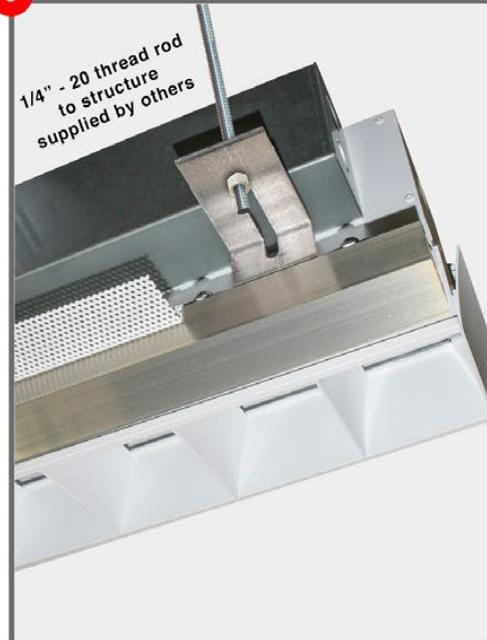
**Step C-** Re-install baffles after housing has been anchored to wall. Make sure inverted V- Shape brackets click into baffles to secure. Add threaded rod from L-brackets to ceiling structure for support.
