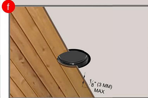
Step E- Install base ceiling and cutout round opening in ceiling to fit around collar diameter. Step F- Start installing panel ceiling over existing base ceiling. Cutout round area for panels to fit and conceal the panel collar.
