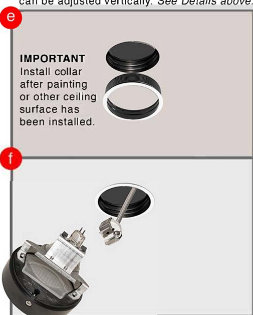
Step E- Flanged collar should be installed after painting, wood, metal ceiling has been prepped. Screw flanged collar into housing. Step F- Hook lamp assembly bi-pin into lamp socket.
