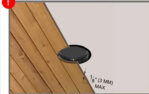
Step E- Install base ceiling and cutout round opening in ceiling to fit around collar diameter. Step F- Start installing panel ceiling over existing base ceiling. Cutout round area for panels to fit and conceal the panel collar.
