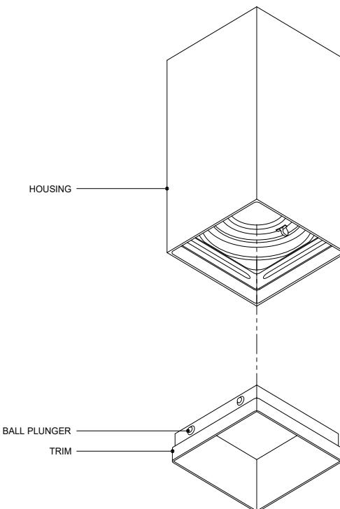
\*\* LED'S SHOULD BE PROTECTED FROM DUST AND DEBRIS DURING INSTALLATION AND MAINTENANCE
