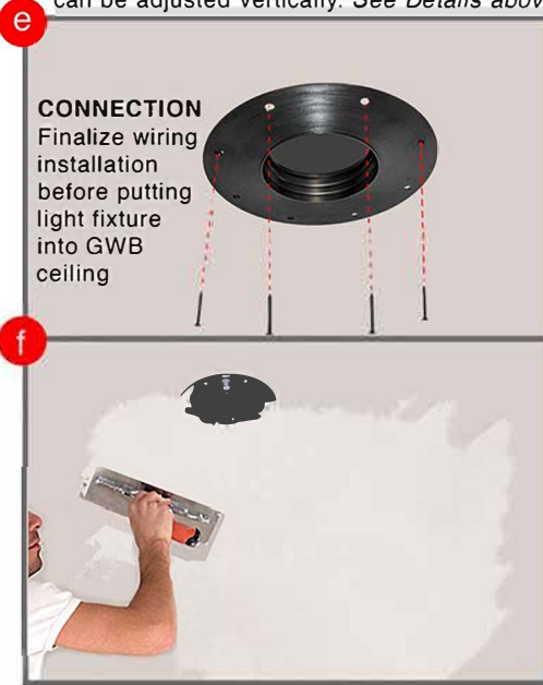
Step E- With Plaster receiver tightly secure against GWB, add GWB screws to further secure plaster receiver. Step F- Apply tape and joint compound (dry). Plaster over ceiling and receiver.
