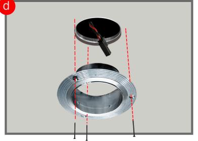
Step D - Thread receiver into collar until plaster flange is snug with the ceiling Step D (optional) - secure receiver with GWB Screws
