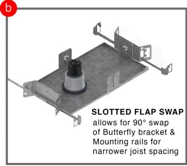
**Step A / B-** Insert mounting rails to brackets. Align bottom of pan to be flush with bottom of joists (no more than 1/8" higher). Slide telescoping rails to meet joist. Fasten to joist with protrusions on rails. If space is limited, Butterfly Brackets can be swapped as shown in Step B.
