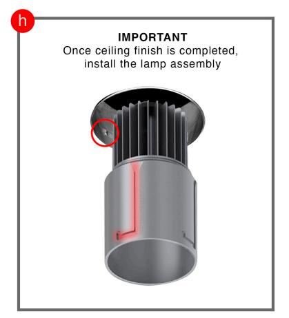
**Step H-** Insert fixture by aligning notches on plaster receiver with J-Hooks on lamp assembly. Turn clockwise to end of travel and let fixture drop into place at bottom of J-Hook feature
