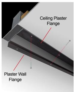
Step 2- Mounting screws go through holes in plaster flanges into wood blocking above ceiling and side wall. Plaster over plaster ceiling flange and wall plaster flange. Paint over dried plaster.
