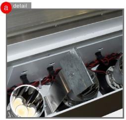
Detail- Closeup showing inverted v- shape metal bracket. Applying pressure on both sides of bracket will release baffle from housing
