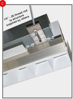
Step C- Re-install baffles after housing has been anchored to wall. Make sure inverted V-Shape brackets click into baffles to secure. Add threaded rod from L-brackets to ceiling structure for support.
