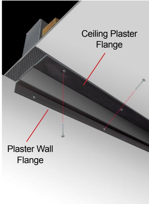
Step 2- Mounting screws go through holes in plaster flanges into wood blocking above ceiling and side wall. Plaster over plaster ceiling flange and wall plaster flange. Paint over dried plaster.
