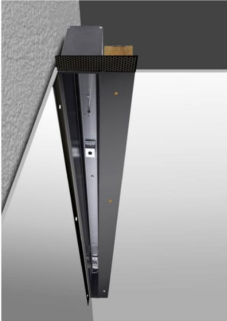
Step 1- Add blocking to support mounting screws. Cut ceiling to fit housing. Fit housing into corner and anchor with mounting screws into top plaster flange and side wall flange.
