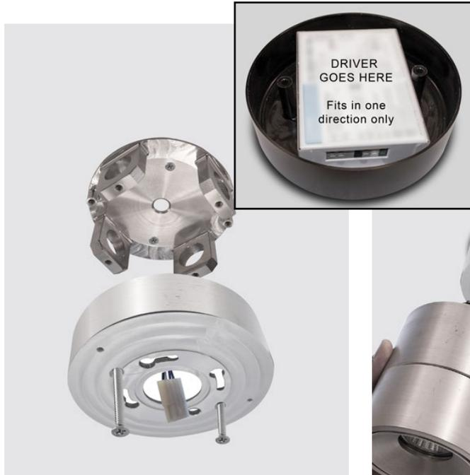
Step 2- Attach Lutron Junction Mounting Driver Box to ceiling plate with #8-32 counter sink screws (Screws supplied by SLI). Driver must be installed before installing Lutron driver box to ceiling.
