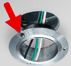
Step 5- Pull power supply and control wires (if required) through ceiling aperture and through the flangeless plaster receiver before threading receiver into J-box mounting hardware. Thread until plaster flange receiver is tight to ceiling. Plaster over mud ring flange, then finish and paint.
